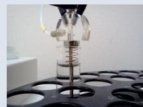
liquid! Usually position one contains activating buffer, position two non-activating buffer and position three a washing buffer (non-activating buffer or another incubation buffer).
